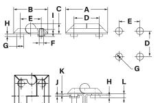
Acid-proof stainless steel external lift-off hinge for flush mounted doors.
