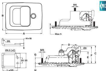
Heavy duty Vector P Slam Action Paddle Latch in black. Flush handle that assembles into your door with a mounting bracket. (Alternative version also available with four mould-in bolts - call for details.)
