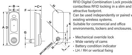
RFID Digital Combination Lock provides contactless RFID locking in a slim and attractive footprint.
