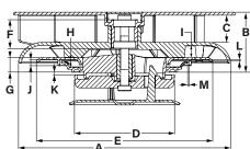
This Rooftop Ventilator is a small, ultra-low profile wind powered ventilator, designed for PLASTIC use on commercial vehicles, pickups, estates, animal vehicles and other applications.
