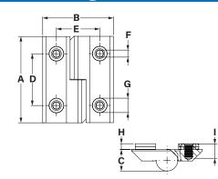
Acid-proof stainless steel external lift-off hinge for flush mounted doors.
