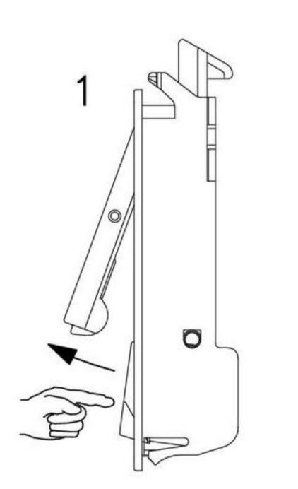
Pressing the trigger button releases the lever and jumps up. The slam latch stays closed.
