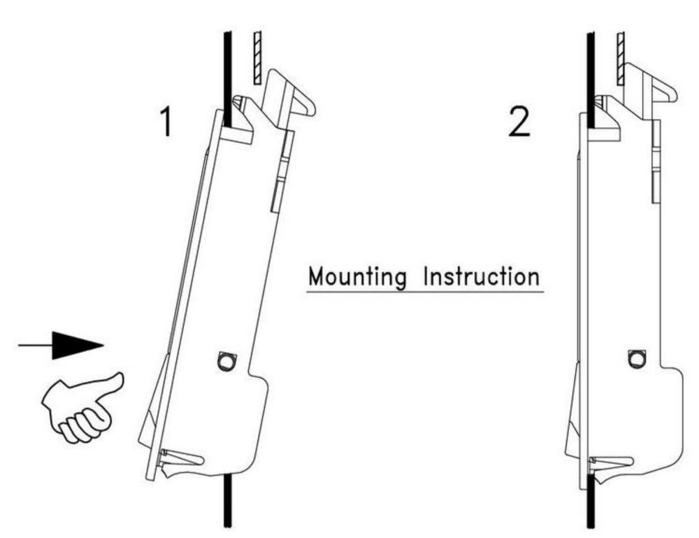
Slide the latch end into the sheet metal....
