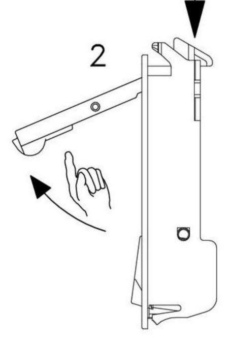
Lifting the lever opens the latch.
