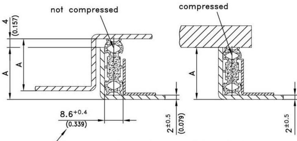
Groove width must not be smaller than 8,6mm(0.339). The best sealing result is only achieved in case the gasket can move freely in the groove and is only hold in position by the 2 central "ears".
