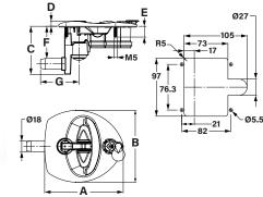
The Vector T handle operates with a 4mm compression feature for a vibration-free closure.
