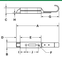
Spring Lock with finger pull latch in zinc plated steel.
