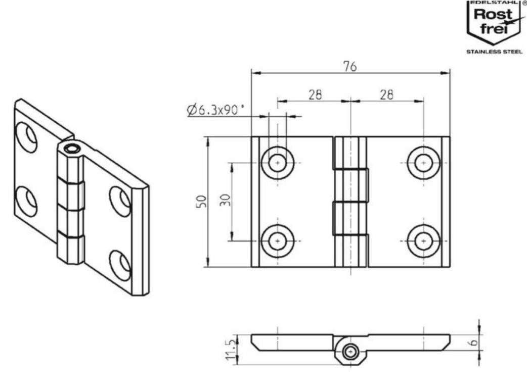
Screw-on hinge AISI 316 for countersunk screw M6
