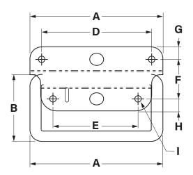
Surface mounted, sprung loaded Drop Handle with plastic cover in mild steel, zinc plated.
