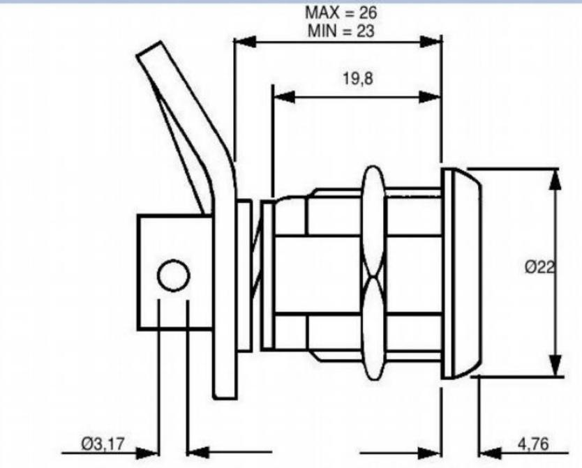
CUSTOMERS CAN FIX CAM IN REQUIRED POSITION WITH A SPLIT PIN
