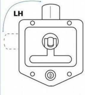
Handle turns anticlockwise to release the latch tongue
