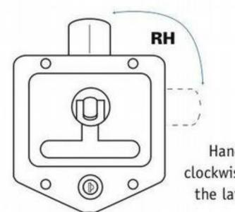
Handle turns clockwise to release the latch tongue
