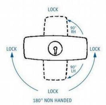
Handles operate through 180° as standard (non-handed). To special order, rotation can be limited to 90° LH (clockwise) or 90° RH (anticlockwise). Handles will lock at each 90° position.
