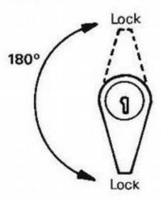
Handles are non-handed and lock in both vertical positions, when key can be withdrawn.
