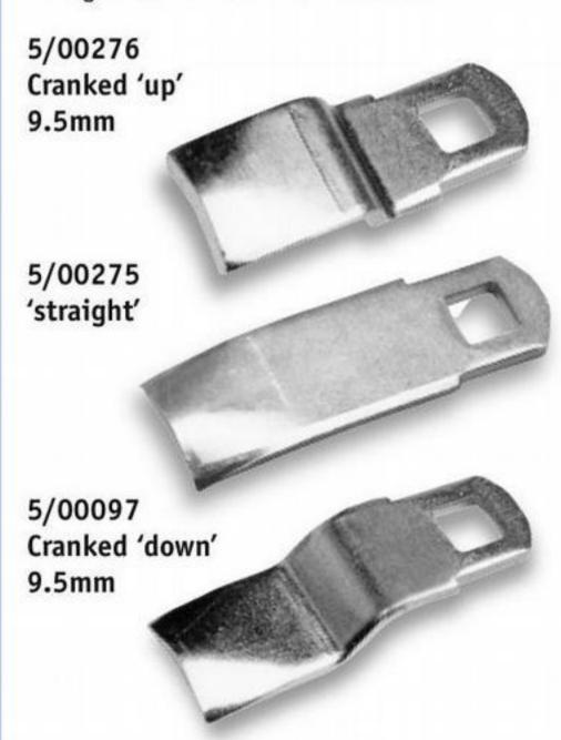
Straight latch bar is fitted as standard, with two options cranked 9.5 mm 'up' or 'down'. Lock will accept all other bars with 8 mm piercing, including 2/3-point options.
