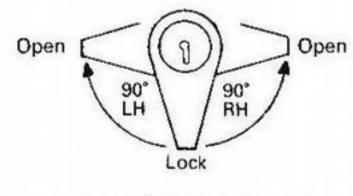
Handles operate LH (clockwise) or RH (anticlockwise) but lock in vertical position only. Key does not withdraw in 'open' position.
