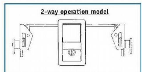
Scheme shows 'paddle' vertical, with two 'claw' latches. Alternatively two slam latches can be fitted, using standard linkage bar (3/12497) at length 915 mm (cut to size). Movement is 13 mm approx., at each side.
