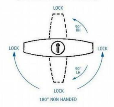
Handles operate through 180° as standard (non-handed). To special order, rotation can be limited to 90° LH (clockwise) or 90° RH (anticlockwise). Handles will lock at each 90° position.
