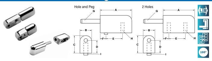
'Block' hinges are a neat, convenient method for hanging externally-fixed doors on metal cabinets, electrical enclosures, etc. Non-handed, the upper part simply sits onto a fixed steel pin. (Oppose hinges for when door is permanently fitted).
